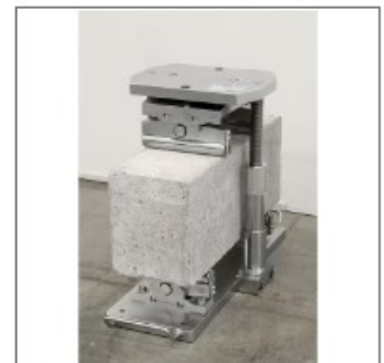
Flexural test device for concrete beams (50-C9010/C)
