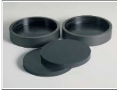
Unbonded caps: steel cap retainers and neoprene pads
